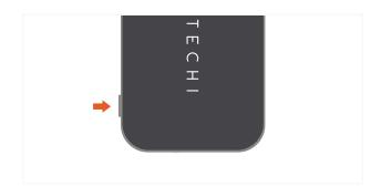
2 Turn on the power bank by clicking the side button once. Once powered on, activate the Apple Watch and Qi charger by double clicking the side button.
