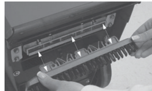
Replacing A Brush
