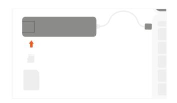
6 Connect up to two data USB devices to adapter's USB-A ports. Max output per port 5V/1A.
