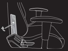
Install the side covers and tighten the bolts. (The covers are marked "L" for the left side and "R" for the
