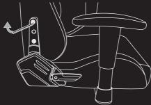
Remove the protective foam covers from the brackets of the seat base. Then position the backrest carefully between the brackets. Insert and attach the 4 bolts (2 on each side) you removed in step 5 by hand rst. Then use the hex key to tighten them. Start with the two bolts on the top of each side, then the bottom two.
