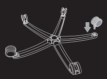
One by one, insert and push the wheels into the base.
