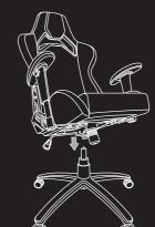
Insert top of the hydraulic lift cylinder into the mounting hole on the control unit, and then turn the chair over in upright position. (Two-person handling required for your safety)
