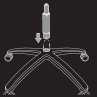
2 Insert the hydraulic lift cylinder into the center hole of the base. Remove the red protective cap on top if there was any
