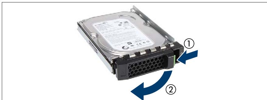
Figure 22: Opening the 3.5-inch HDD module locking lever
