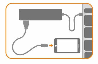
**6.** All ports can be used simultaneously. *Output of each USB Type-A port is 5V / 1A*
