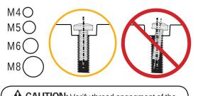
**A** CAUTION: Verify thread engagment of the screw or spacer/screw combination in STEP 1-2. — Too short will not hold the  $\mathsf{TV}$
