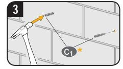
Insert two anchors C1 (Fischer UX8x50R included in Concrete Anchor Kit CMK3\*).
