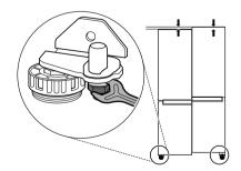
Open the door and use the spanner ① to loosen the keeper nut by turning it to the left.
