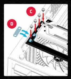
After installing the GPIU in to motherboards PCI-E slot, affix the bar to the case and GPU using the (C) four M6-32 screws and the (D) metal plate.
