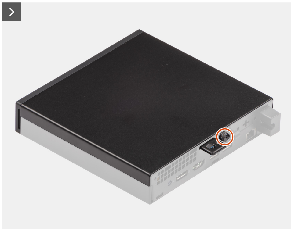
Figure 9. Removing the side cover
