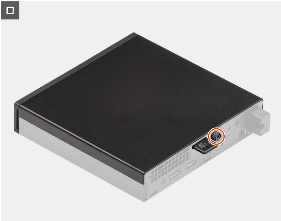
Figure 12. Installing the side cover
