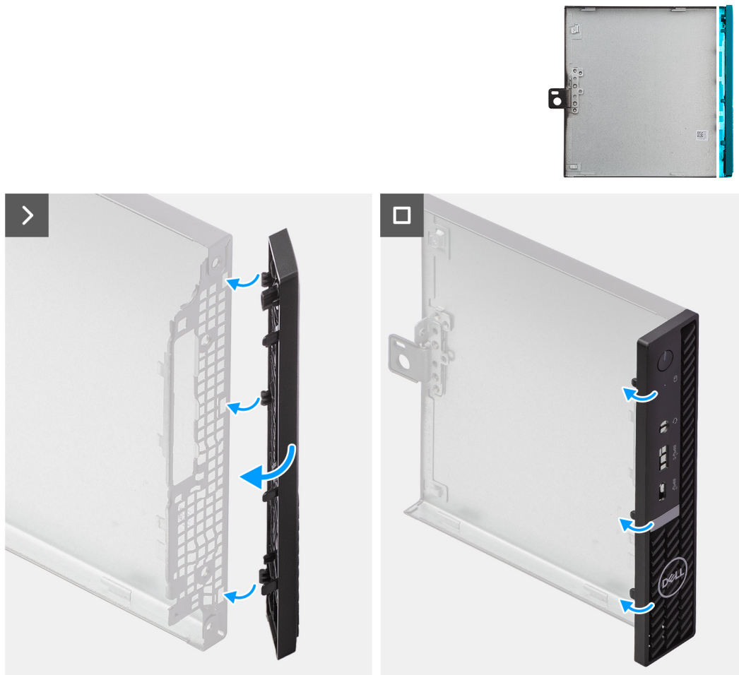
Figure 16. Installing the front bezel
