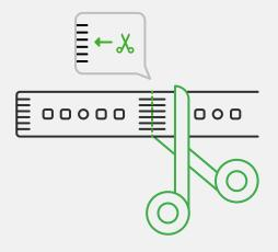
**NOTE:** Once cut, the strip cannot be connected back together, so ensure you've measured properly before cutting.
