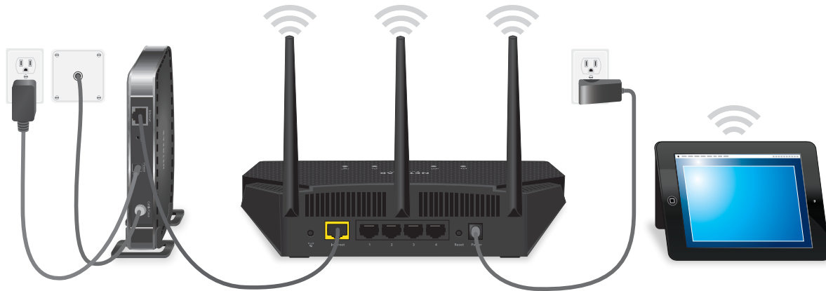
Figure 4. Connect the access point in default router mode to your modem
