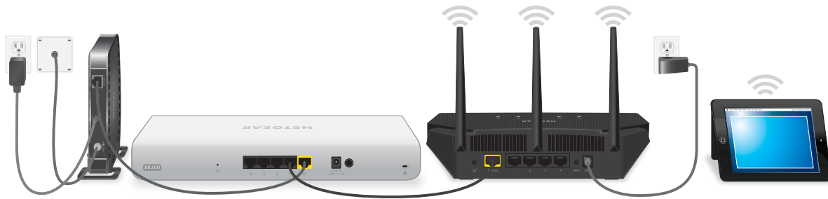
Figure 5. Connect the access point to an existing router in your network
