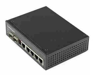
Easily deploy or scale your network with this Gigabit Ethernet switch, features four dedicated PoE+ enabled ports, and one dedicated open SFP slot plus the flexibility of a switchable RJ-45/Open SFP port for use as an uplink or for non-PoE devices. It features an IP-30 housing, compact design, and is wall and DIN rail mountable.
