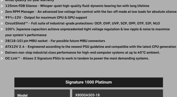
At 20%/50%/100% load AC 115V Internal, the power **Efficiency** efficiency should be at least 90%/92%/89% **Protection** OCP/OVP/UVP/SCP/OPP/OTP/SIP/NLO **Output Capacity** 1000W **Operation Temperature** 0~40°C Regulatory CB,CE,FCC,BSMI, TUV, cTUVus, 3C, RCM 135 x 135 x 25 (mm) FDB Silent Fan Fan
