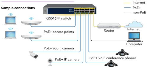
Note: This switch is designed for indoor use only. If you want to connect to a device located outdoors, the outdoor device must be properly grounded and surge protected, and you must install an Ethernet surge protector inline between the switch and the outdoor device. Failure to do so can damage the switch.
