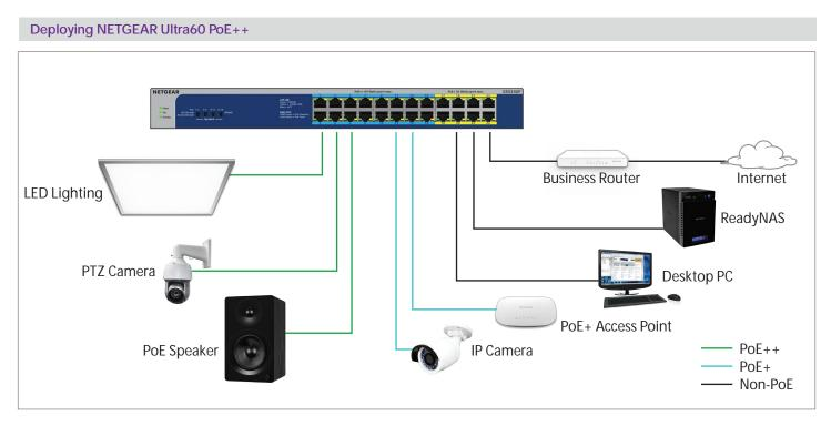
GS516UP and GS524UP can support, but are not limited to, power the devices shown in the above examples.
