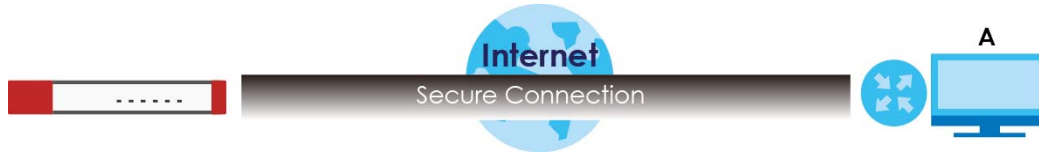
Figure 551 SSH Communication Over the WAN Example
