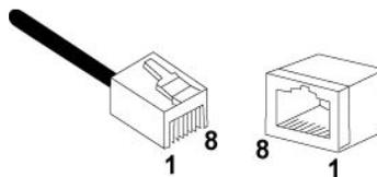
Figure 23. RJ45 Connector and Port Pin Layout
