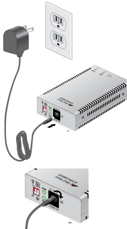
Figure 22. Connecting 12VDC Powered Unit
