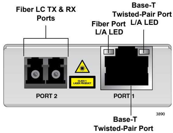
Figure 12. MMC2000/200LC Series and AT-MMC2000/LX/LC Front Panel
