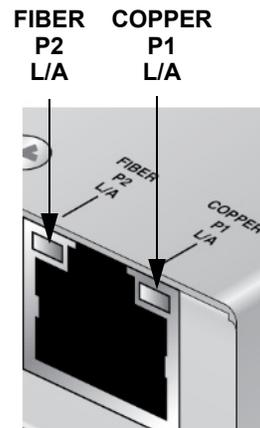
Figure 2. Port LEDs
