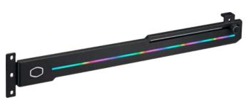
A smart add-on GPU brace to protect your graphics card and motherboard for longer period of use. The Cooler Master ELV8 helps reduce the sag of heavier graphics cards and the stress on PCI-e slot on the motherboard. The length and height adjustments allows it to work with almost any graphics card. It also features a beautiful addressable RGB strip to enhance the light sync with the entire system.
