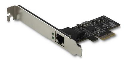
This single-port 2.5Gbps PCIe network card offers a versatile and low-cost way to deploy 2.5GbE network connectivity. It adds one copper Ethernet port to your server or desktop computer and provides Multi-Gigabit Ethernet access to your network at four speeds: 2.5 Gbps, 1G, 100Mbps, 10Mbps.
