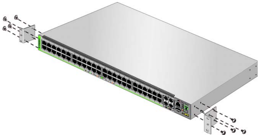
Figure 21. Example of Attaching the Brackets to the Switch
