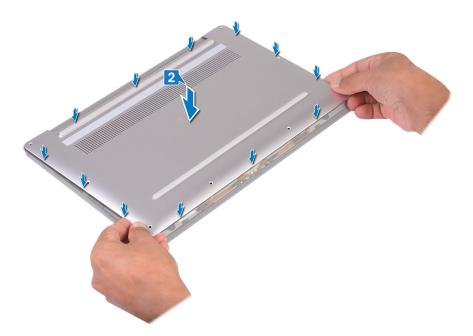
3 Replace the eight screws (M2x3, Torx) that secure the base cover to the palm-rest assembly.
