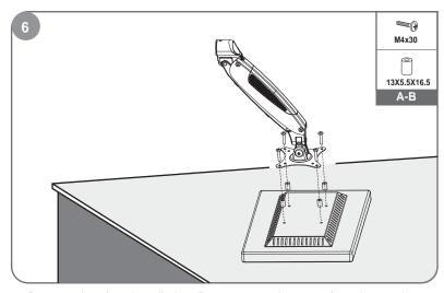
Recessed surface installation: Put 4 spacers between faceplate and monitor. Install 4 screws through faceplate, spacers to monitor via mounting holes.
