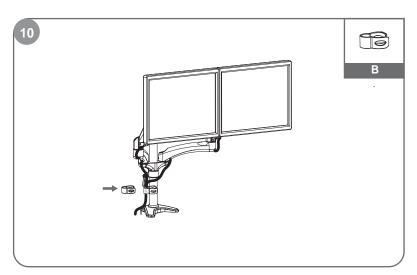
Insert cables into cable covers.
