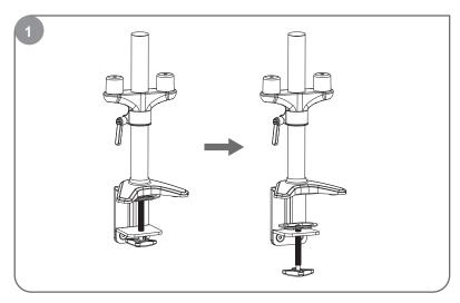
Loosen clamp screw until enough space is left for the edge of the desk.
