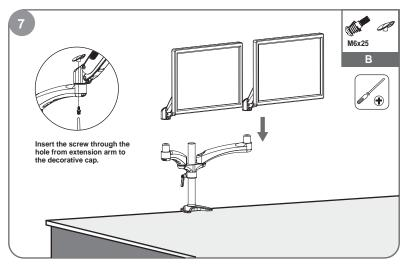
Lift the spring arm along with the monitor and put it on the extension arm.
