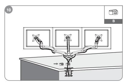
Insert cables into cable covers. Leave enough slack of cables at arm joints for fully adjustment.
