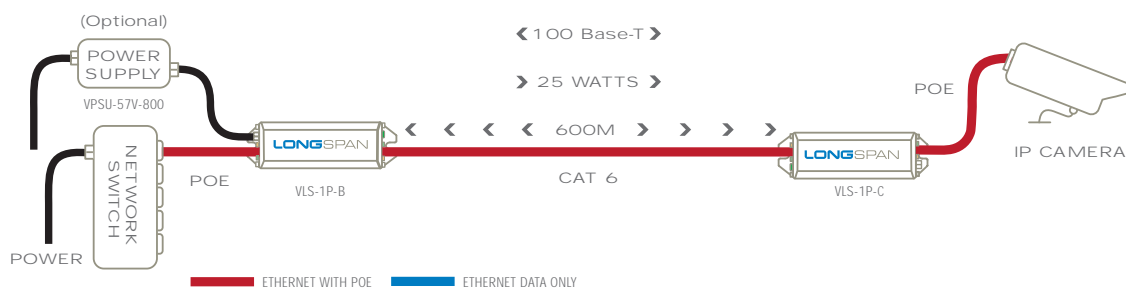
Diagram 1. A pair of LONGSPAN converters deliver full-bandwidth Ethernet & optional full-power POE over greatly extended distances of regular network cable or UTP.
