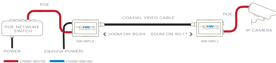
Diagram 1. HIGHWIRE Powerstar delivers Ethernet and POE over legacy coax, for maximum reliability with minimal wiring.
