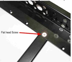
9. Once the cross braces are rmly attached, the completed unit can be mounted into the cabinet/rack. The cable manager is mounted at the same time and is simply placed over the rack mounting brackets then both are fastened to the rack posts.
