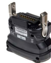
1139-01-SO-MC9X00-CAC TSL Common Access Card reader for MC9100
