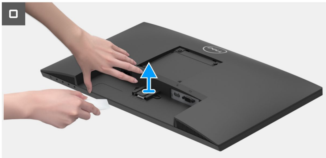
Figure 12. Removing the back cover
