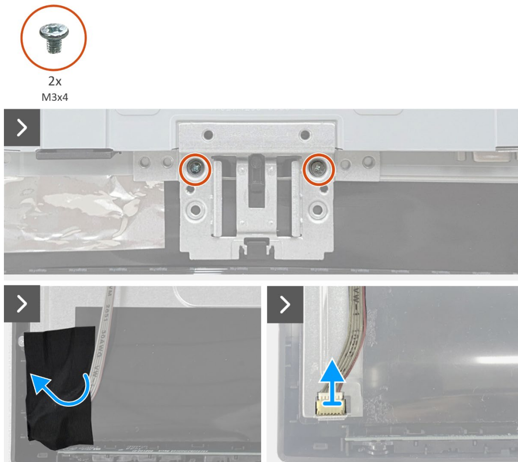
Figure 16. Removing the chassis assembly
