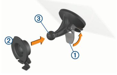
2 Press the mount 2 onto the suction cup ball 3 until it snaps into place.
