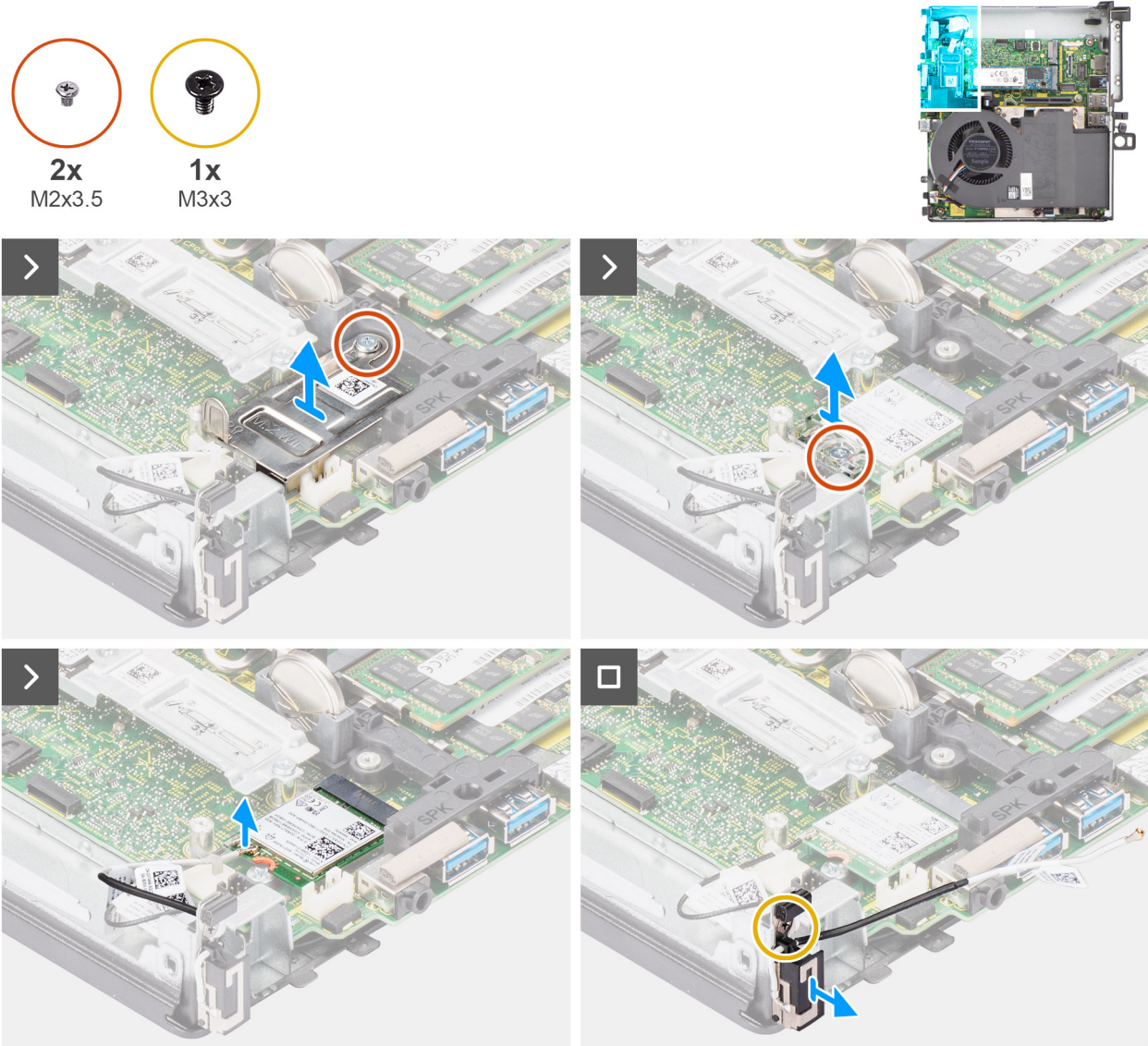
Figure 52. Removing the internal antenna—location 1
