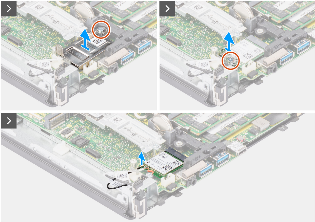
Figure 54. Removing the internal antenna—location 2
