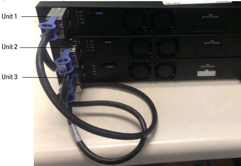
Figure 1-6. Connecting a Stack of Switches
