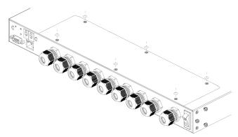
2. Remove the cover from the compartment and loosen the cable gland by turning the gland nut counter-clockwise (use a dedicated spanner if required).
