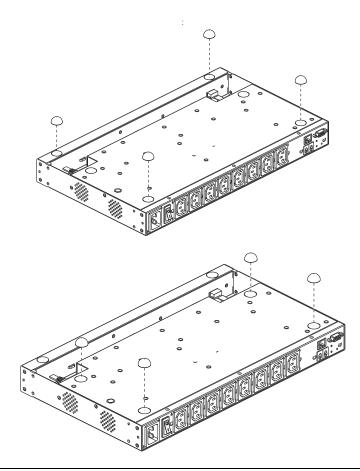
**Note:** To ensure adequate ventilation, allow at least 5.1 cm on each side, and 12.7cm at the back for power cord and cable clearance.
