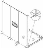
3. Line up the plastic corner caps (#4) with the holes on the corners of the panels. Use the M3 (8 mm) at-head Phillips screws (#6) to attach the corner caps (#4) to each of the eight corners on the rack.
