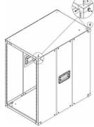
4. Turn the rack on its side and use the bracket screws (#11) to attach the casters (#9) (#10) to your rack.
