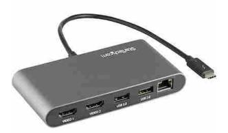
This certified Thunderbolt 3 docking station is a compact mini dock, delivering essential connections for productivity. The bus-powered dock connects dual 4K HDMI displays, Gigabit Ethernet, and two USB-A (USB 3.2 / 2.0) ports and for flexible set up, the attached Thunderbolt 3 cable has an extended length of (11 in./ 28 cm).
