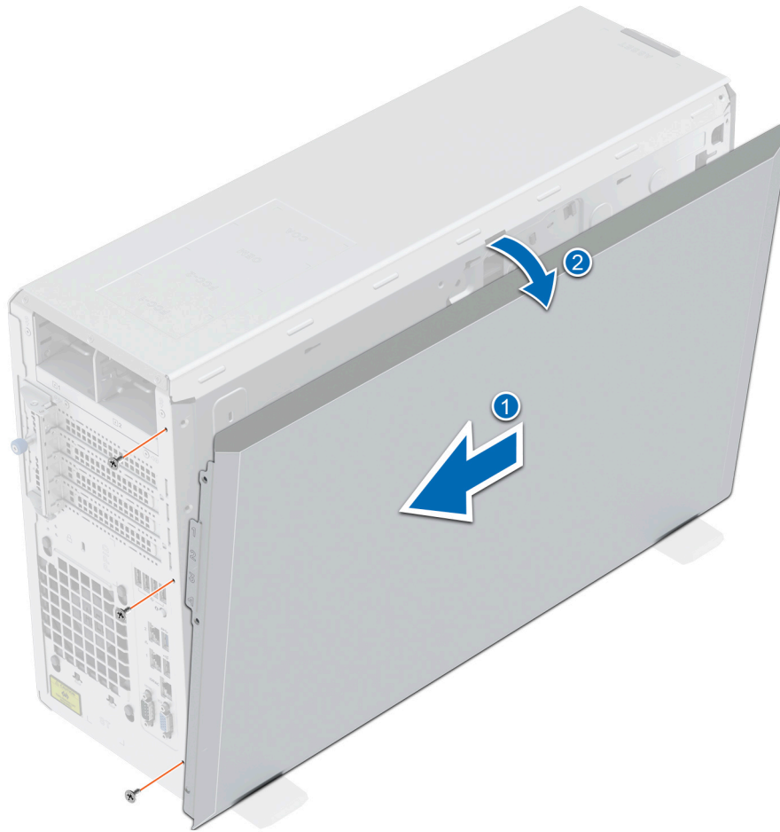
Figure 94. Removing the system side cover
