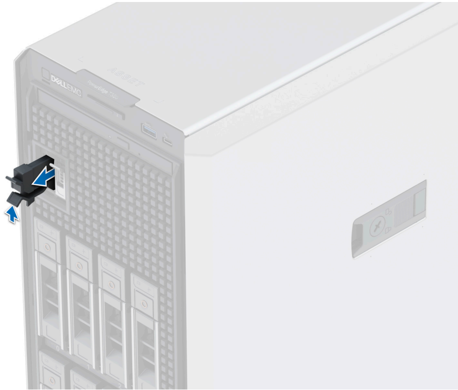
Figure 61. Removing the BOSS S2 card carrier blank
