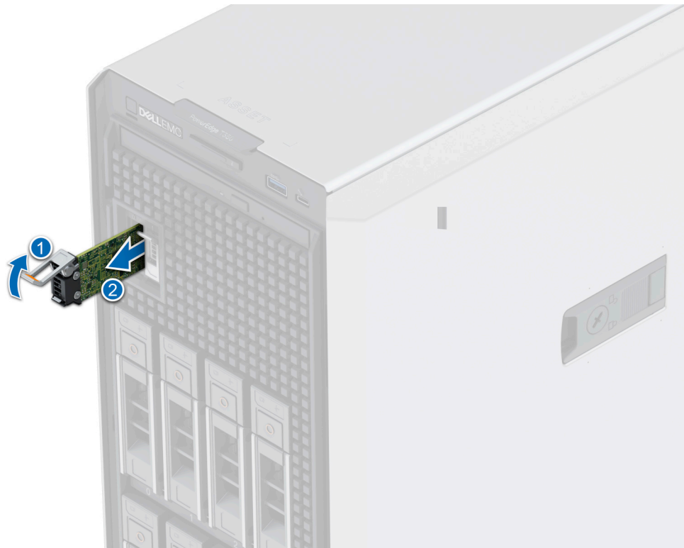
Figure 63. Removing the BOSS S2 card carrier
