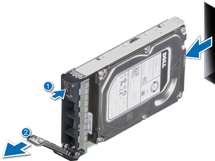
Figure 24. Removing a drive carrier
