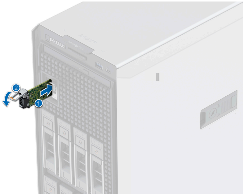
Figure 70. Installing the BOSS S2 card carrier
