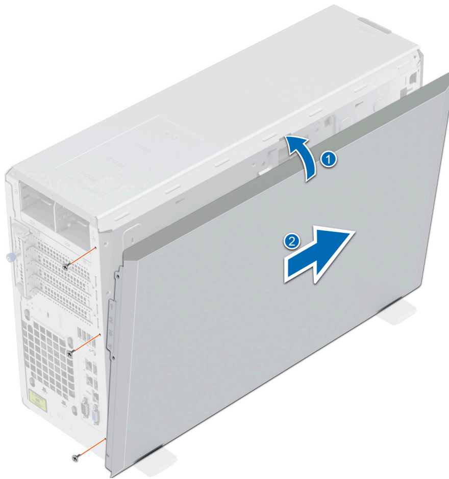
Figure 101. Installing the system side cover
