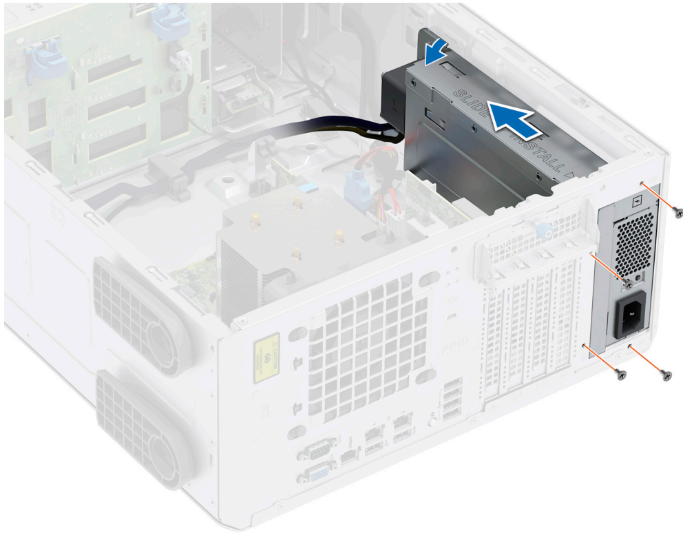
Figure 81. Removing the PSU cage
