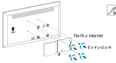
**Note:** The Spacers (J) are optional. They may be necessary if the VESA Mounting Points at the back of the Monitor are recessed.
