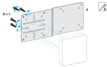
**Note:** Use two Screws on either the vertical or horizontal Short Mounting Slots.
