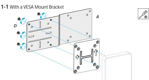
**Note:** Use the speci c Screws and VESA Mount Bracket that came with the NUC or Thin Client.
