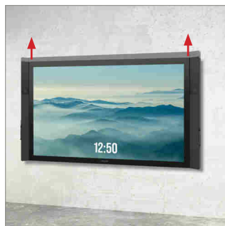
Interface arms include height adjustment screws to help level the screen.
