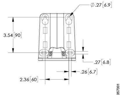
Figure 13: L-bracket AP mount dimensions
