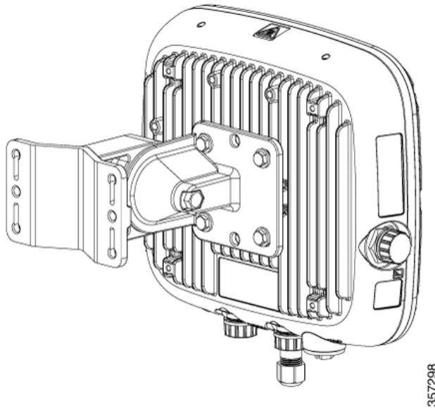
**Figure 7: Pivoting Wall Mounting Bracket**
