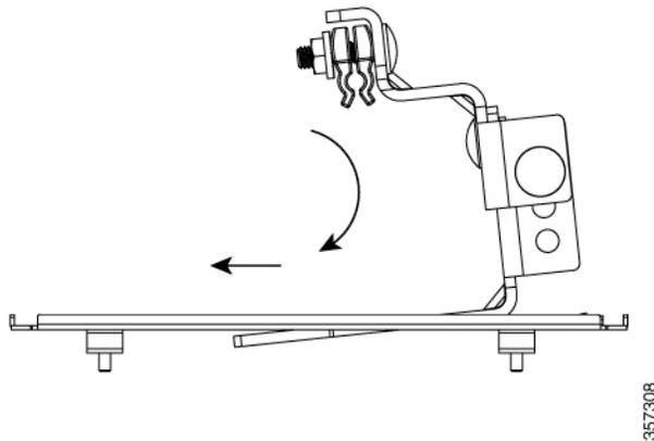
**Note** If needed, reposition the AP on the bracket assembly so it hangs level. Loosen the M8 screws just enough to move on a slotted hole, then re-tighten the screws to 15 lbf-in (17 kgf-cm) of torque.
