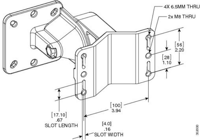
**Figure 9: Exploded View of the Pivoting Mounting Kit**
