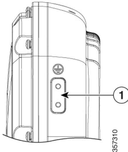
1 Ground pad, where the ground strap screw holes are located.
