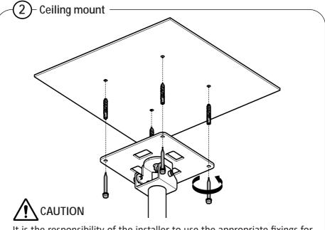
It is the responsibility of the installer to use the appropriate fixings for the specific installation location.
