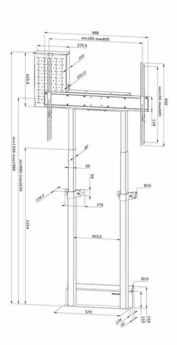
Neomounts Measuring unit: mm
