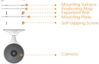
Step1 Drill screw holes on the mounting surface as the mounting map shows, and then put in the expansion bolts.
