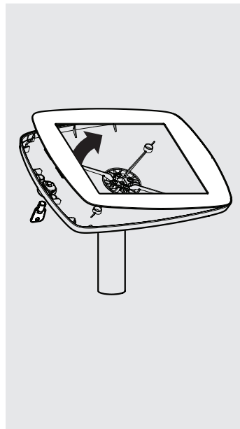
2 Unlock & remove the Faceplate from the Bouncepad Case.
