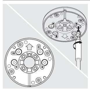
Con gure the angle of rotation - ensuring both arrows are pointing in the same direction before starting. Default angle con guration is 270°. Insert the limit screws for 90° or 180° rotation.
