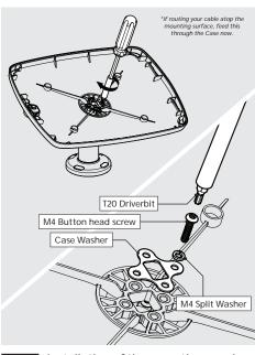
Installation of the mounting arm is complete. Now install your Case as shown above.
