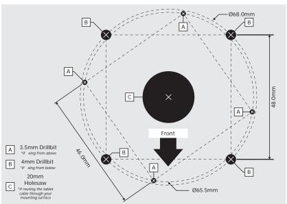
4 Use the above template to mark the drill holes - appropriate to your chosen xing method. 'A' if xing from above. 'B' if xing from below. Follow the corresponding steps (PTO) specied to each xing method.
