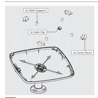
Install the Tablet Setup Kit. Each kit is speci c per tablet device and Bouncepad Case.
