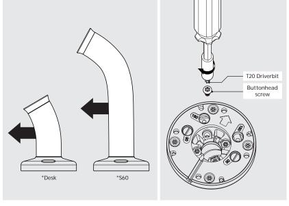
Attach your chosen mounting arm. Your mounting arm must forward lean in the same direction as the two arrows. Tighten by hand, ensuring full and correct engagement.
