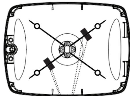
Use the adhesive cable clip to secure cable in the nearest quadrant to the Tablet Power Port
