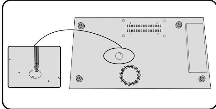
The machine is supplied with a thermal re-set switch. The switch will activate when the machine becomes too hot. This condition should not occur during normal use. To re-set the switch:
