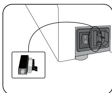
This machine is fitted with a fuse, located between the main switch and the wall socket on the rear of the machine. To replace the fuse:
