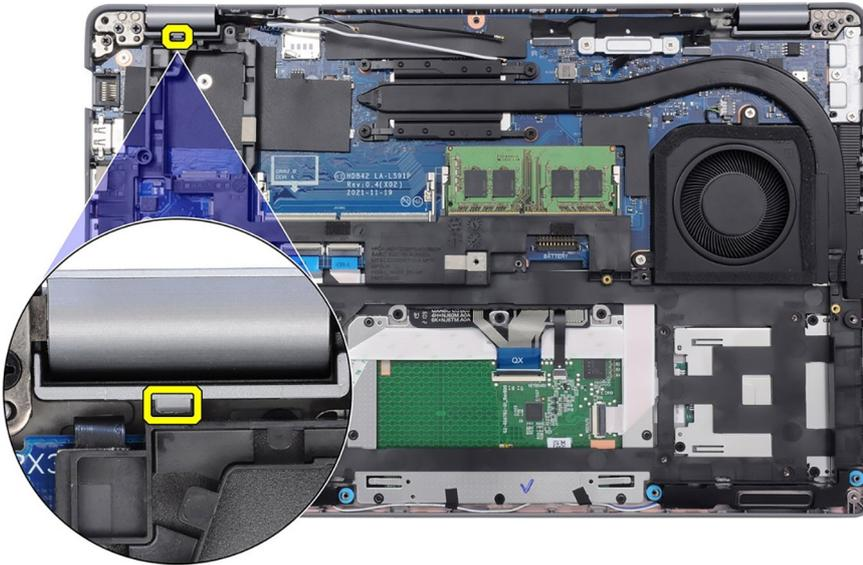
2. Replace the ten (M2x3) screws that secure the assembly inner frame to the system board and the palm-rest assembly.
