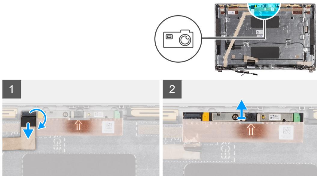
Figure 1. Removing camera module
