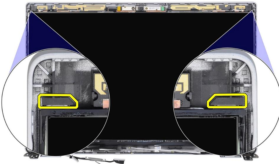
2. Lift and open the display panel to access the display cable.
