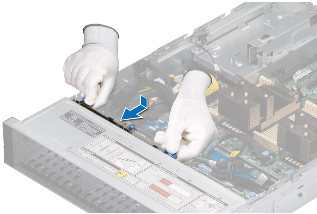
Figure 50. Installing the drive backplane
