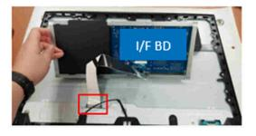
S15 Unlock / screws on 56 7 C3,89 ( ee Red mark'
