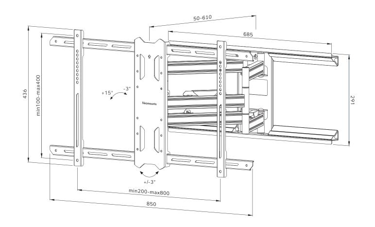
Neomounts Measuring unit: mm
